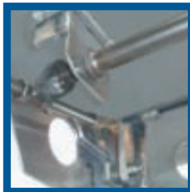
Steel latching mechanism for tailgate
